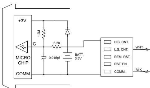
Moving the white wire to the "H.S. CNT." Input allows the CUB Counter to operate at speeds up to 5 KHz when driven by bi-polar outputs or external circuits having an output impedance of  $3.3 \text{ K}\Omega$  or less. Input drive voltage must be limited to 3.0 V maximum to avoid damage to the counter. Outputs higher than 3.0 V can be used with an external voltage divider, as shown.
