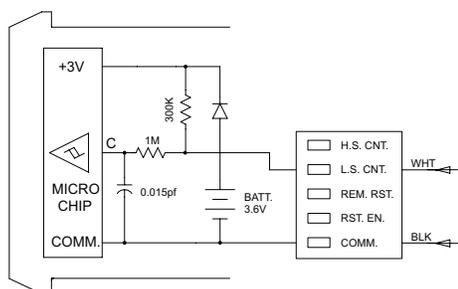
Pulling the "L.S. CNT." Input to Common with a mechanical or solid-state switch increments the counter. The low pass filter (*1 meg resistor and 0.015 pf cap*) used with a Schmidt trigger circuit debounces mechanical switch signals. The switch load is  $14 \mu\text{A}$  (*max. voltage drop 0.5 V*) when ON. OFF-state leakage current must be less than  $2 \mu\text{A}$ .
